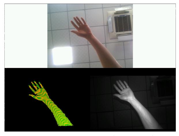
The pictures above show three images on RK3288 screen (1536x2048), from top to bottom and left to right, they are RGB, DEPTH, IR respectively. The size are all 640x480, in which the depth image displays the disparity image in RGB565 format directly.
